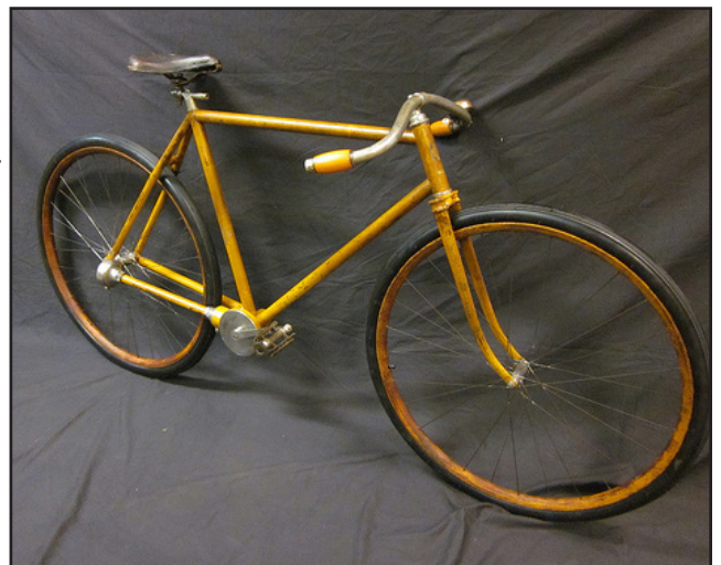
The Yellow Fellow Racer. Note the wheels are wood and it is a chainless drive.
