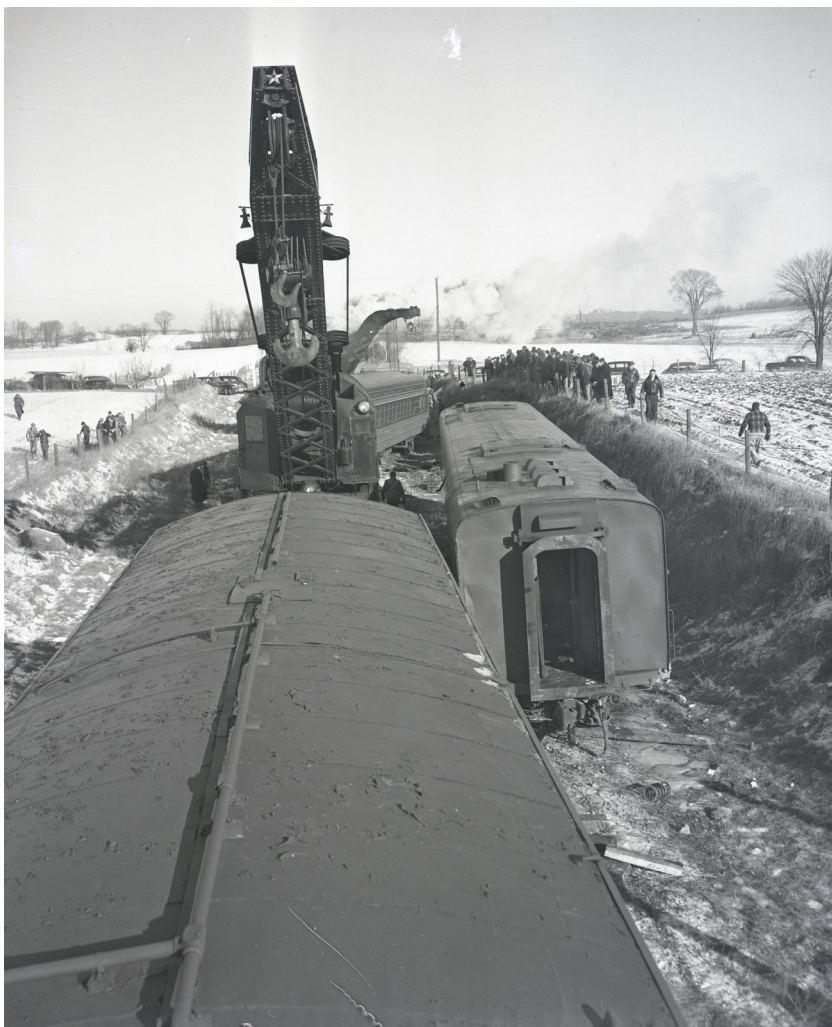
The Milwaukee and Green Bay wreckers combine to lift the damaged Beaver Tail car back onto the repaired rails at Meadowlark Road. The Diner-Lounge 5252 is at the right.
