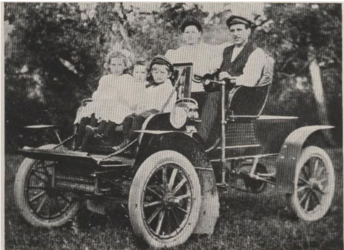
The two cylinder, four passenger "Brotz Special" made by Mr. Brotz in 1902-1904 from his own designs. Motor and parts were turned out on a foot power lathe. All parts—chassis, post steering apparatus, transmission, rear axle—were made at home. Mr. Brotz is at the wheel with Mrs. Brotz. The Brotz children occupy the front "rumble seat."
